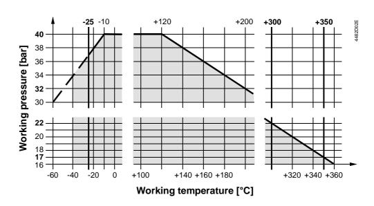
Working pressure staged as per ISO 7268 and EN 1333 at operating temperatures of -25 ... +300/350 °C as per DIN 4747 and DIN 3158.
