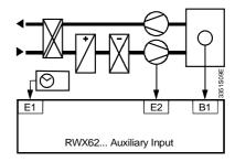
**"Standby" operation:** [ $\bigcirc$  STNDBY]. On switching an AC 24 V signal (e.g., fan OFF message) to binary input **E2**, the control loop is switched to a zero output state excepting the frost protection function.
