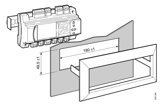
Electrical installation You can use normal cables for wiring the POLYGYR system. However, when mounting in an extremely impaired EMC environment, use only shielded cables.
