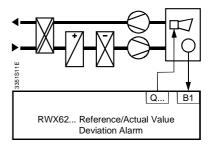
For each controller, one common deviation alarm contact is available for all active sequence control loops. The alarm function can be deactivated by entering an extreme setting for the corresponding DEVALM setpoints.
